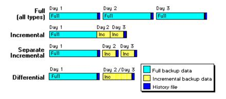
To show how the three basic backup methods deal with changed files (as indicated by the archive bit), assume your hard disk had only four files (A, B, C, D) that had just been backed up using the Full method. As your files change in the days that follow, each method would back up different files to the data set. The Full method backs up all files, the Incremental method backs up files as they change, and the Differential method backs up changed files cumulatively:
